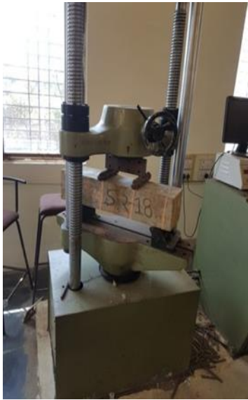
Fig 2 Testing of beam specimen under three point loading in UTM machine
